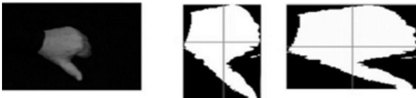
Figure 4. Trimming process and Scaling normalization applied to input image.
