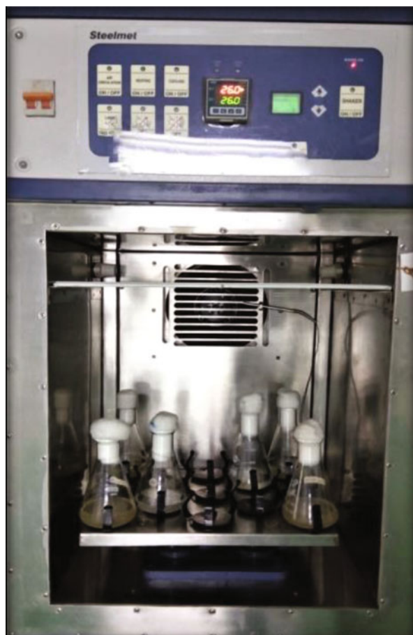
Fig. 10.3 Shaking cooling incubator used for plant cell suspension culture
