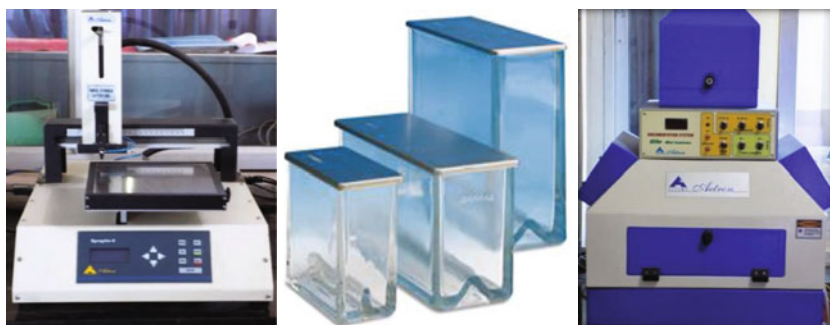
Fig. 5.1 HPTLC automatic sample applicator, Chromatography chambers and documentation system for TLC visualization and analysis
