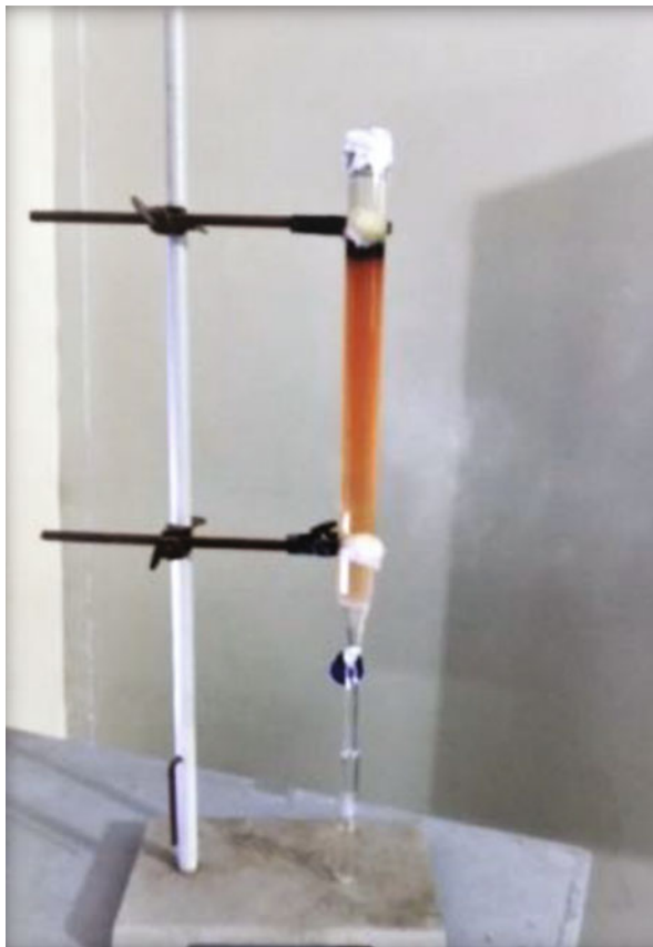
Fig. 5.3 Silica gel column used for activity-guided separation
