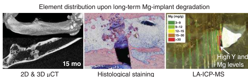
Figure 5.10 LEFT: 3D (upper) and 2D (lower) \mu CT scans for long-term bone response implants. Middle: Histological staining to assess local tissue response. Right: LA-ICP-MS analysis showing chemical image of implanted Mg pins, from which relative mass was calculated for assessment of degradation rates. Source: From Amerstorfer et al. [105]/with permission of Elsevier.
