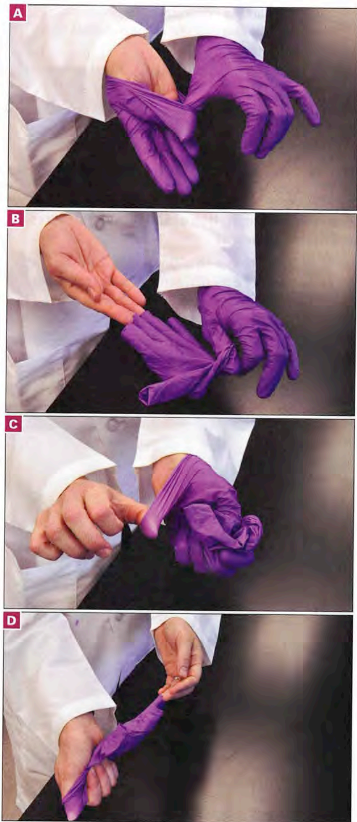
FIGURE S.4 Proper Glove Removal • Protective gloves fit tightly around the hands and must be removed in such a way that limits their snapping, which produces aerosols. (A) Begin by hooking the thumb of one hand under the cuff of the glove on the other hand. (B) Next, roll the glove off the hand so that it turns inside out. (C) Take the removed glove in the hand that still has a glove on it and repeat the process. (D) As you roll the second glove off your hand, the first glove will end up inside the second glove, which also ends up inside out. Upon completion, all contaminated surfaces are inside the second glove.
