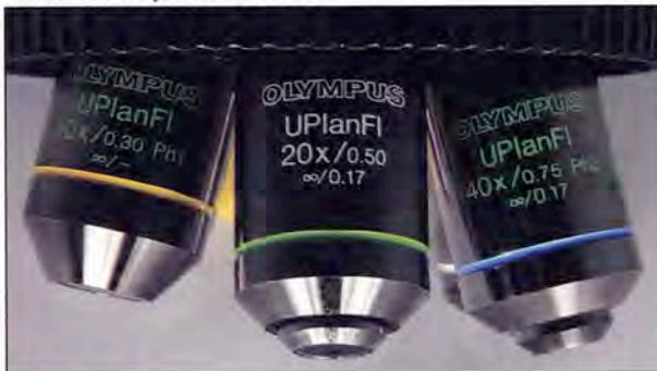
FIGURE 1.3 Lens Magnification Markings • The markings on an objective lens barrel describe the lens' optical features. Here we focus on magnification markings. Objective Lenses: The yellow-banded lens provides a 10\times magnification; the green-banded lens provides a 20\times magnification; and the blue-banded lens provides a 40\times magnification. These color bands are standard for quick magnification reference. Many microscopes also have a 4\times lens, which would have a red band (not shown). Oil-Immersion Lens: This lens has two bands; the white band indicates the lens provides 100\times magnification; and the black band indicates this lens must be used with immersion oil to obtain the sharpest image. Note that the word oil is also etched on the lens' barrel. Immersion oil can damage lenses that do not have an “oil” specification. Ocular Lens: The lens shown here provides a 10\times magnification. Some ocular lenses are not 10\times , so check the specifics before calculating final magnification.
