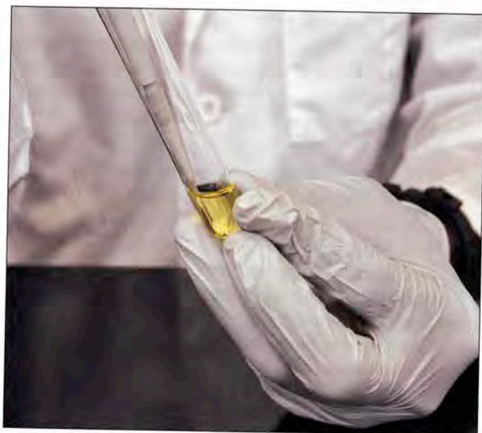
FIGURE D.5 Dispensing to a Liquid • Hold the pipette on a slight angle with the tip immersed in the liquid and held against the glass of the test tube (or plastic of a microtube). Press the control button gently to the first stop (don't shoot out the liquid!). When no more fluid comes out, continue pressing to the second stop to completely empty the pipette. Remove the pipette along the glass (plastic), then slowly release pressure on the control button and replace the cap on the test tube. Eject the tip into a biohazard container if transferring a culture (Fig. D.6).
