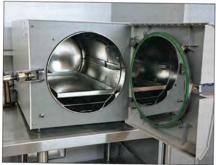
FIGURE S.7 An Autoclave • Media, cultures, and equipment to be sterilized are placed in the basket of the autoclave. Steam heat at a temperature of 121°C (produced at atmospheric pressure plus 15 psi) for 15 minutes is effective at killing even bacterial spores. Some items that cannot withstand the heat, or have irregular surfaces that prevent uniform contact with the steam, are sterilized by other means.
