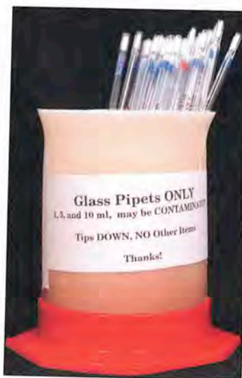
FIGURE C.8 Dispose of the Pipette • The pipette must be disposed of correctly, especially if it is contaminated with microbes. Each lab has its own specific procedures, and your instructor will advise you what to do. Shown here is a jar used for reusable glass pipettes. Disposable pipettes must be placed in an appropriate biohazard container. In either case, be careful when removing the pipette from the mechanical pipette. There is danger of culture dripping from the pipette or of breaking the glass or plastic.
