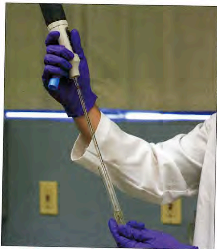
FIGURE C.7 Filling the Pipette • Carefully draw the fluid into the pipette. Briefly bring it to a vertical position and read the volume. Notice how the tube's cap is being held by the pinky finger of the pipette hand.
