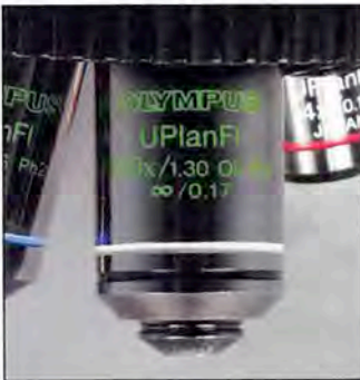
FIGURE 1.3 Lens Magnification Markings • The markings on an objective lens barrel describe the lens' optical features. Here we focus on magnification markings. Objective Lenses: The yellow-banded lens provides a 10\times magnification; the green-banded lens provides a 20\times magnification; and the blue-banded lens provides a 40\times magnification. These color bands are standard for quick magnification reference. Many microscopes also have a 4\times lens, which would have a red band (not shown). Oil-Immersion Lens: This lens has two bands; the white band indicates the lens provides 100\times magnification; and the black band indicates this lens must be used with immersion oil to obtain the sharpest image. Note that the word oil is also etched on the lens' barrel. Immersion oil can damage lenses that do not have an “oil” specification. Ocular Lens: The lens shown here provides a 10\times magnification. Some ocular lenses are not 10\times , so check the specifics before calculating final magnification.
