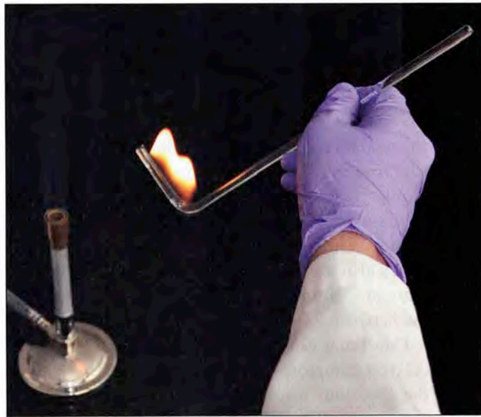
FIGURE 5.3 Flaming the Glass Rod • Dip the glass spreader into some alcohol and then flame the spreader to burn off the alcohol.
