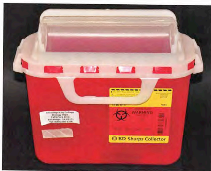
FIGURE S.5 Sharps Container • Needles, glass, and other contaminated items that can penetrate the skin or an autoclave bag should be disposed of in a sharps container. Do not fill above the dashed black line. Notice the autoclave tape in the lower left. The white stripes will turn black after proper autoclaving. Above the autoclave tape is the address of the institution that produced the biohazardous waste.
