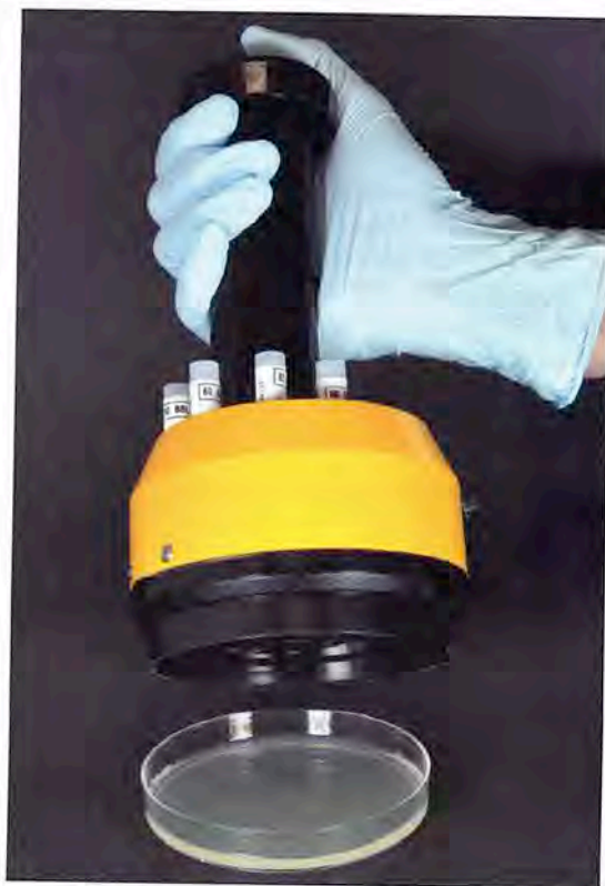
FIGURE 43.1 Disk Dispenser ■ A disk dispenser, like the one shown, is sometimes used to uniformly deposit disks on a Mueller-Hinton agar plate.
