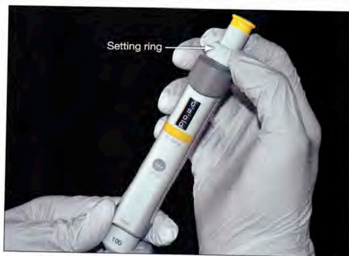
FIGURE D.2 Setting the Volume • Rotate the adjustment knob (setting ring) to set the volume on a micropipette. This pipette has been set at 90.0 \mu L (the line between the last two zeroes is a decimal point). Never rotate the adjustment knob beyond the volume limits of the pipette as it may become damaged.
