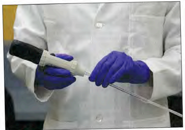
FIGURE C.6 Assembling the Pipette • Carefully insert the pipette into a mechanical pipette. Notice that the pipette is held near the end with the fingertips. For safety, the hand is out of the way in case the pipette breaks.
