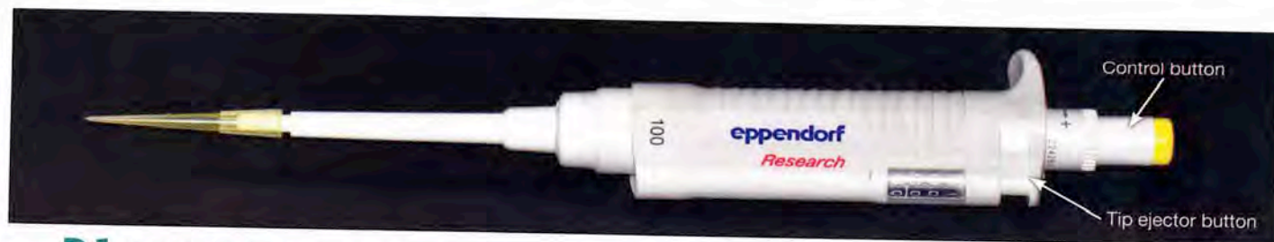
FIGURE D.1 Micropipette • This is a micropipette that dispenses volumes between 10 \mu L and 100 \mu L. Also, always use a micropipette with the appropriate tip. As shown here, tips and pipettes are often color-coded. If the tips have been sterilized, always close the tip case when not picking up a tip.
