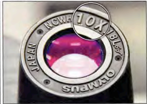
FIGURE 1.3 Lens Magnification Markings • The markings on an objective lens barrel describe the lens' optical features. Here we focus on magnification markings. Objective Lenses: The yellow-banded lens provides a 10\times magnification; the green-banded lens provides a 20\times magnification; and the blue-banded lens provides a 40\times magnification. These color bands are standard for quick magnification reference. Many microscopes also have a 4\times lens, which would have a red band (not shown). Oil-Immersion Lens: This lens has two bands; the white band indicates the lens provides 100\times magnification; and the black band indicates this lens must be used with immersion oil to obtain the sharpest image. Note that the word oil is also etched on the lens' barrel. Immersion oil can damage lenses that do not have an “oil” specification. Ocular Lens: The lens shown here provides a 10\times magnification. Some ocular lenses are not 10\times , so check the specifics before calculating final magnification.
