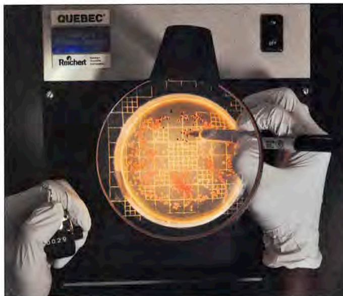
FIGURE 10.3 Counting Bacterial Colonies • Place the plate upside down on the colony counter. Turn on the light and adjust the magnifying glass until all the colonies are visible. Using the grid in the background as a guide, count colonies one section at a time. Mark each colony with a felt-tip marker as you record with a hand-tally counter.
