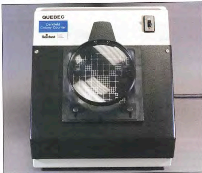
FIGURE 6.5 Colony Counter • A colony counter provides magnification and transmitted light to help us see subtle differences in colony shape and size. However, colony color and many other features are best determined with reflected light. The grid in the background is a counting aid; each big square is 1 square centimeter.
