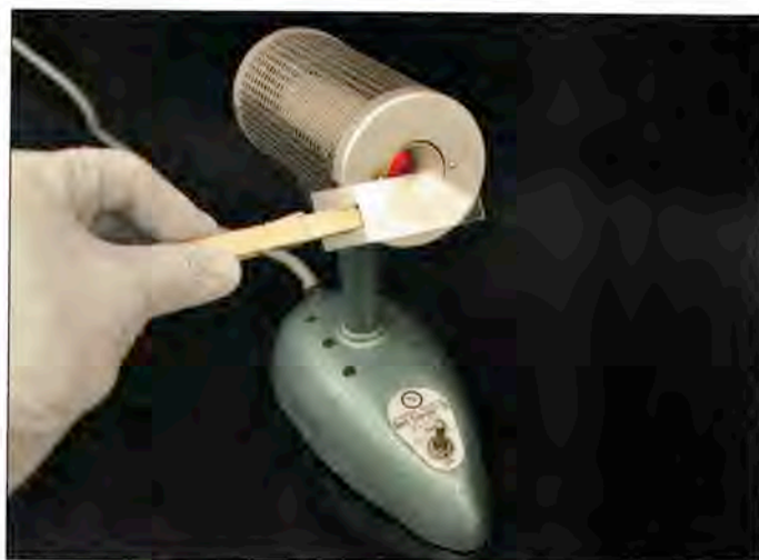
FIGURE 11.5 Heat Fixation Using an Incinerator • To heat fix a slide using an incinerator, hold the slide near the microincinerator's opening (with the smear facing away from the opening) for 5–10 seconds.
