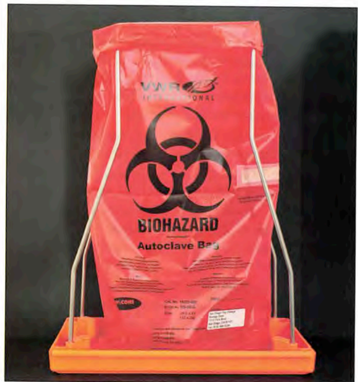
FIGURE S.8 An Autoclave Bag • Nonreusable items (such as plastic petri plates) are placed in an autoclave bag for decontamination. Petri plates should be taped closed. Do not overfill or place sharp objects in the bag. Notice the autoclave tape at the middle right. The white stripes will turn black after proper autoclaving. At the lower right is the address of the institution that produced the biohazardous waste.
