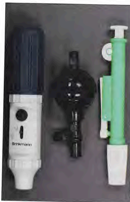
FIGURE C.1 Mechanical Pipettes • Three examples of mechanical pipettes are shown here, each with its own method of operation. Your instructor will show you how to properly use the style of pipette available in your lab. From left to right: A semi-automated pipette, a pipette bulb, and a plastic pump.
