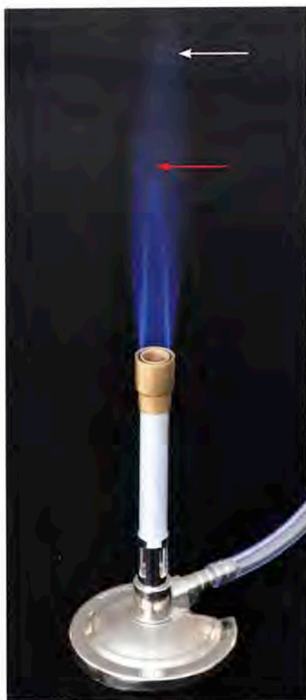
FIGURE 3.10 Bunsen Burner Flame • When properly adjusted, a Bunsen burner produces a two-cone flame. The inner cone (red arrow) is the hottest and is where the inoculating tool wire is inserted for sterilization. The outer cone (white arrow) is used to heat the mouths of open glassware items.
