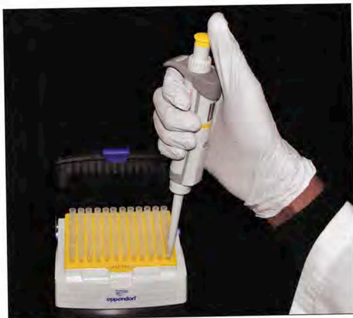
FIGURE D.3 Micropipette Tips • Micropipettes must be fitted with a (sterile) tip of appropriate size (often color-coded to match the pipette). Open the case and press the pipette into a tip, then close the case to maintain sterility. Do not touch the pipette tip.
