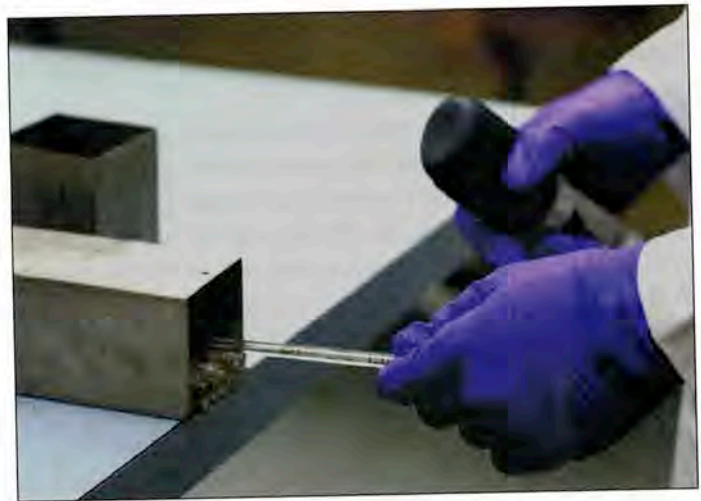
FIGURE C.5 Getting the Sterile Pipette • Pipettes of the same size are autoclaved in canisters, which then are opened and placed flat on the table for stability. Pipettes are removed as needed by only touching the end opposite the tip.
